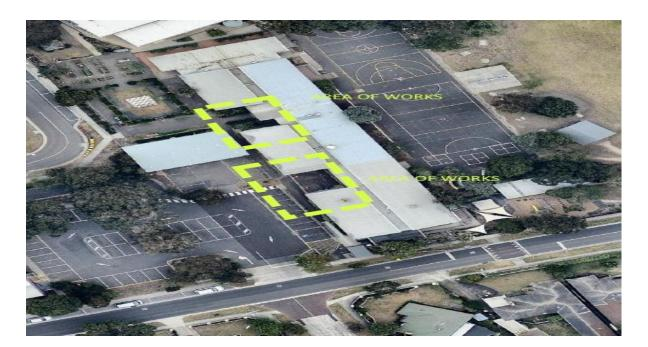
The main school building is single storey, timber framed construction with thin block cladding battened onto the timber frame. The building has a timber floor supported by concrete stumps and a metal sheeting roof supported by open web steel roof trusses. It was indicated that the building is approximately 60 years old.
